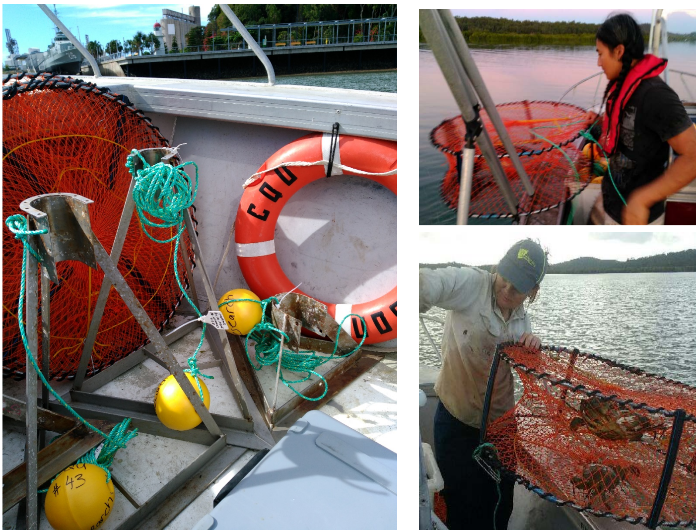
Figure 1: Sampling equipment used for mud crab monitoring: heavy duty crab pots and steel frames in two sizes for BRUVS (cameras were mounted at the apex, pointed downwards at a bait bag attached to the centre of the base).
