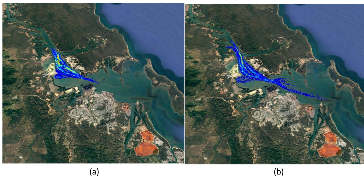
Figure 3.2: CONNIE estimates of the dispersal of silt from the eastern side of the bund wall in Western Basin for releases on (a) the 1 of July 2015 and (b) the 1 January 2016. The results are visualised in Google Earth with dark red indicating that > 5% of released particles travelled through the cell, whereas dark blue indicates less < 1%.
