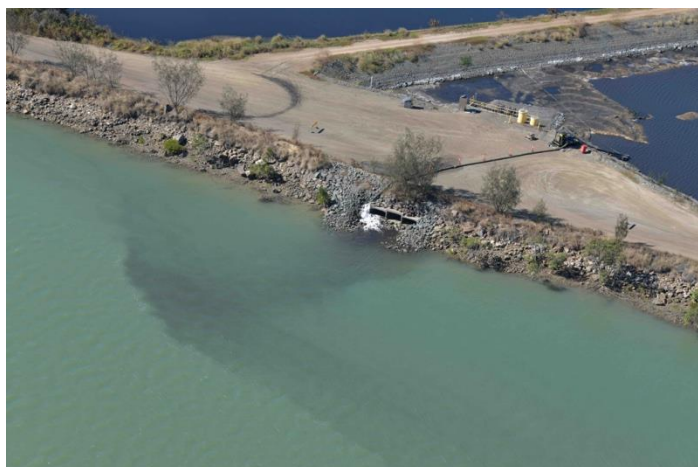
Figure 26. Black discolouration in Calliope River estuary associated with pump effluent from the coal loading facility site—Calliope estuary, Zone 6.
